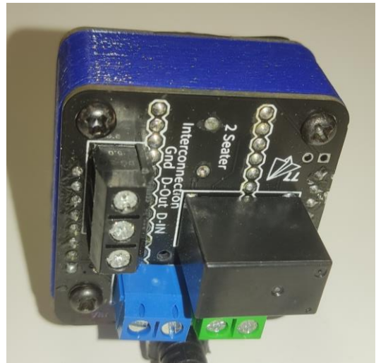
instrument panel mounted controller (encoder + 3x pushbuttons) Labelling not applied as yet
