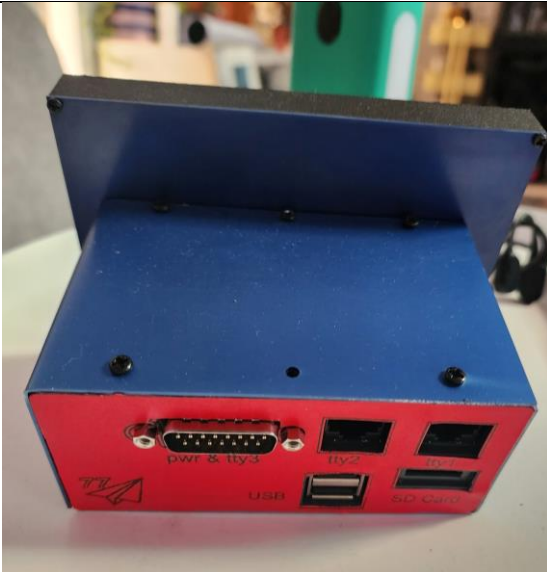
Power, coms, usb and sd card connections/interface
